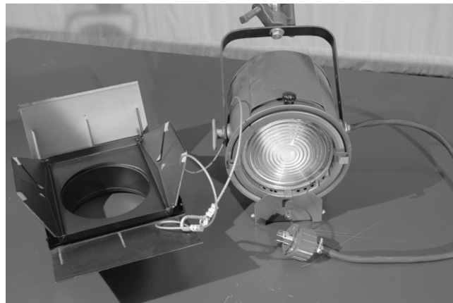
Photo 5.3 The Fresnel spotlight has a lamp, reflector, lens, and a focusing knob for controlling the spread of the light beam it produces. It comes in a variety of wattages, depending on production needs. Notice the set of barn doors , or black metal flaps, used to block light from parts of the studio where it is not wanted.
