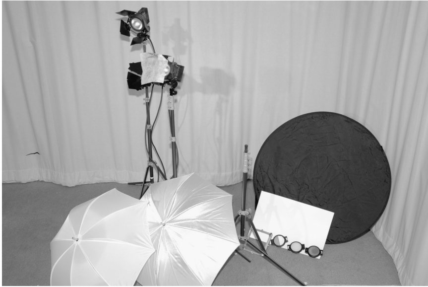
Photo 5.9 Some of the typical contents of a field lighting kit: portable lights clipped to their stands, reflector umbrellas, a flag (the black circular item to the right), a white balance card, filters (three are visible leaning against the card), and extension cords.
