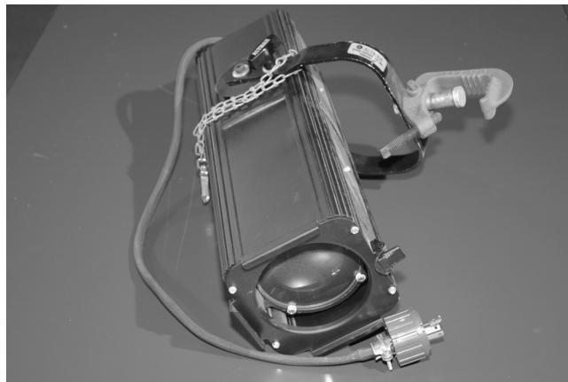
Photo 5.4 The ellipsoidal spotlight produces a well-defined beam that can be further shaped with metal pattern inserts. In this photo, the C-clamp used to affix the instrument to the lighting grid is clearly in view, as is the lamp's safety chain , used to further ensure that the lamp stays where it belongs.
